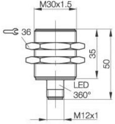
**Inductive Sensors** BES M30MF-USC15B-S04K M30x1.5 x 50 normally-open Sn=15mm shielded
